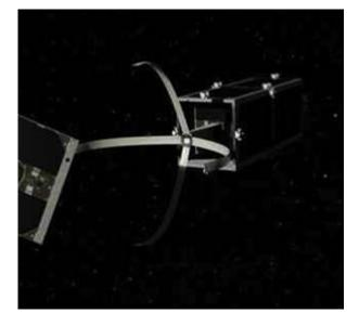
A proposed Swiss satellite to deorbit cubesats is one of several technologies being proposed or developed to clean up orbital debris, which could have additional economic benefits as well. (credit: EPFL)
